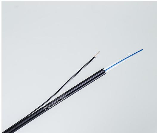
The toneable micro flat drop cable is engineered for last-mile FTTH deployments requiring a compact, lightweight, and highly durable optical drop solution. The cable incorporates a single optical fiber buffered to 0.9 mm and housed within a UV-resistant polyethylene jacket formulated for long-term outdoor performance.
